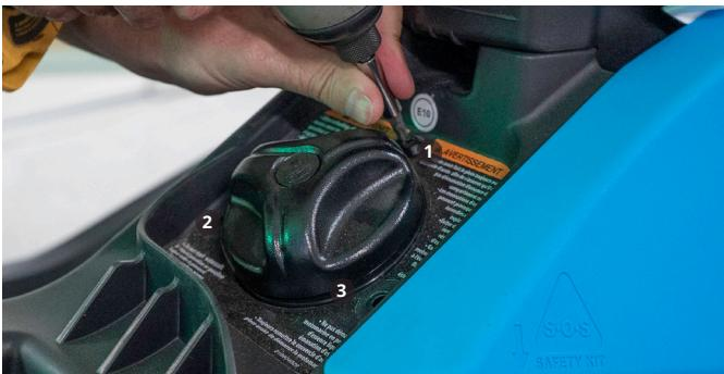
4. Remove the torx bolt located under the panel at the front of the steering and remove the panel.
