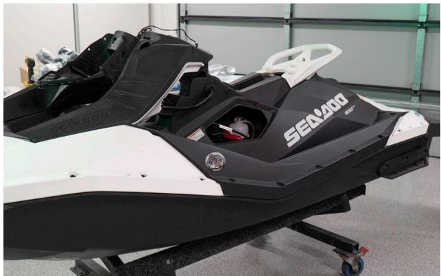
14. Remove the hull lifting up and toward the front of the ski so that the steering arm slides through the grommet.
