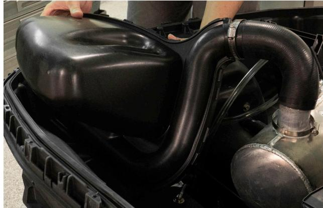
**22.** Sikaflex the rim of the outlet. Ensure an ample amount is used.
