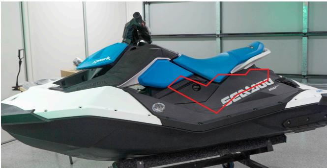
3. Undo the 3 x Torx bolts near the tank.
