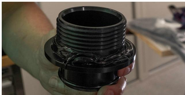
**23.** From the inside of the hull, place the outlet through the OEM outlet position with the thread facing outside.
