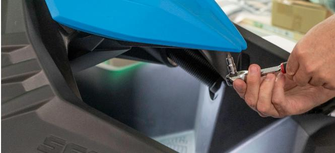
5. Undo the steering clamp by removing the 2 x 10mm bolts.
