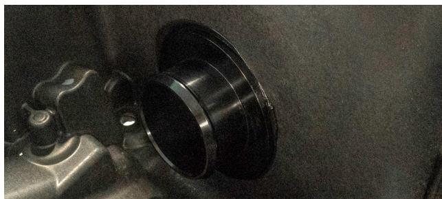
**23.** Attach the provided silicone hose and resecure hose clamps.
