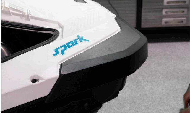
**16.** Undo the 16 torx bolts on the white plastic around the rear of the ski.
