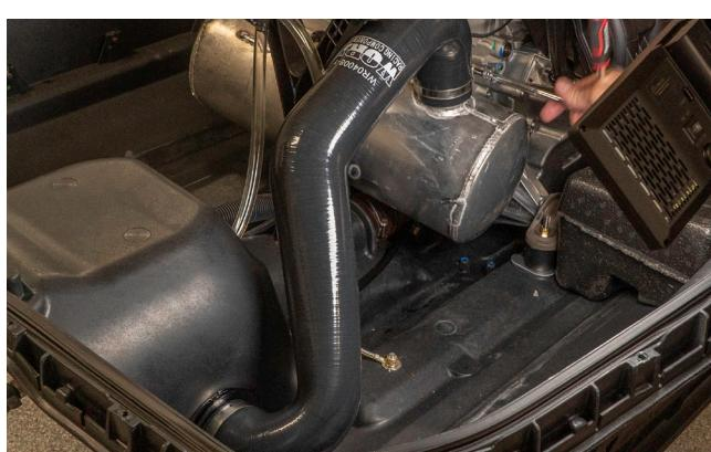
**24.** Attach the lock nut from the pump tunnel and tighten.
